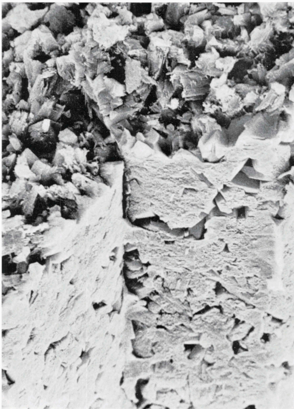
Fig. 33. Wood sample 117: francolite; Carboniferous; Foy, France. Scanning electron micrograph of oblique radial section, showing coarsely crystalline surfaces and cleavage planes of tracheid casts, 5250 X, TFDL.
