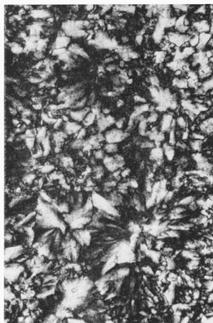
Fig. 12. The same section as in Fig. 11 with crossed nicols, showing hyperblastic crystallization, same enlargement.
