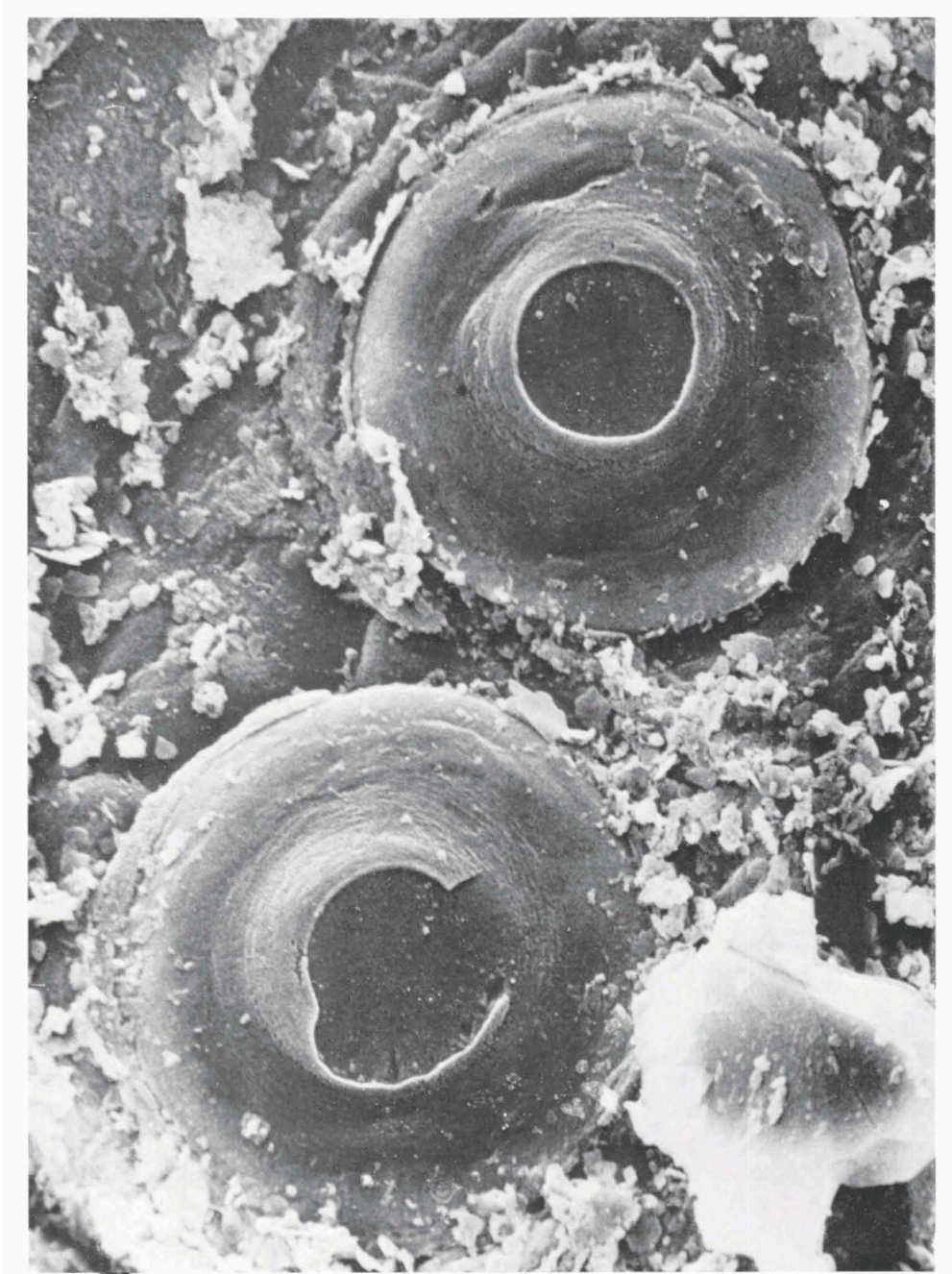
Fig. 37. Wood sample 97: disordered tridymite + quartz; age and origin unknown. Scanning electron micrograph of a tangential wall of a tracheid, showing two bordered pits with a concentric fibrillar structure at the surface, 3850 X, TFDL.
