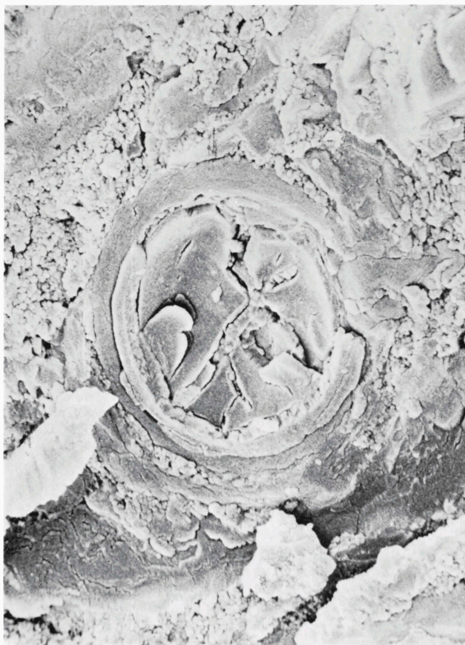
Fig. 19. Wood sample 88: quartz; age and origin unknown. Scanning electron micrograph of a radial section, showing a collapsed bordered pit, 5250 X, TFDL.
