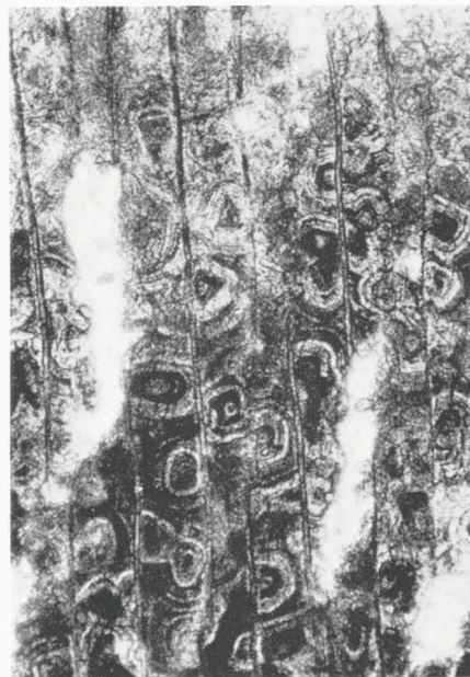
Fig. 31. Wood sample A25: goethite + lepidocrocite; Pleistocene; Ugchelen, The Netherlands. Oblique radial section, normal light, 100x. Faint tracheid walls and accretion lines of ferric nodules.
