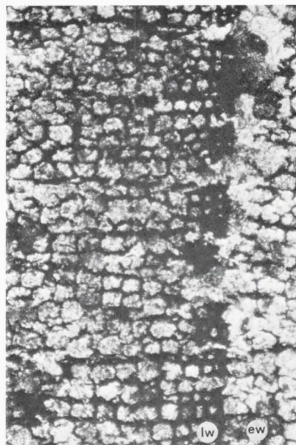
Fig. 23. Wood sample 70: siderite; age unknown; Siegen, Germany. Cross-section, crossed nicols, 100x. Sideritic matrix with lignitic remains of cell walls (ew = early wood; lw = late wood).
