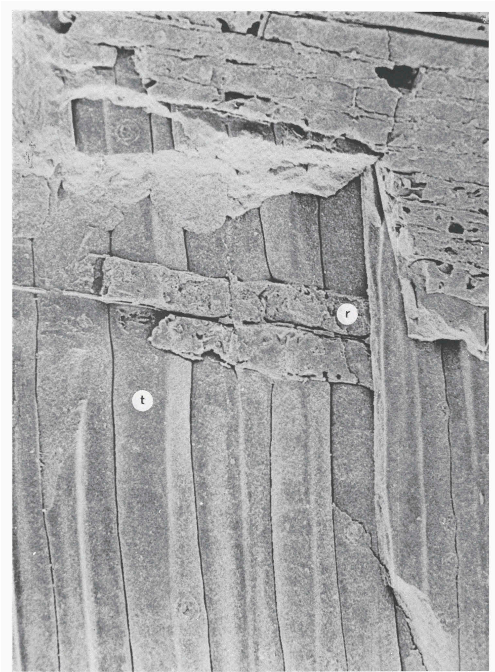
Fig. 16. Wood sample 168; quartz; age unknown; Moscow, U.S.S.R.; RGM 159 992. Scanning electron micrograph of a radial section, 437.5 X, TFDL. Smooth structures with ghosts of bordered pits.
