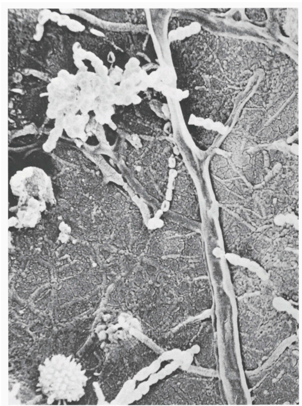
Fig. 36. Wood sample 176: goethite; age and origin unknown. Scanning electron micrograph showing hyphae and spores of fungi, 5250 X, TFDL.
