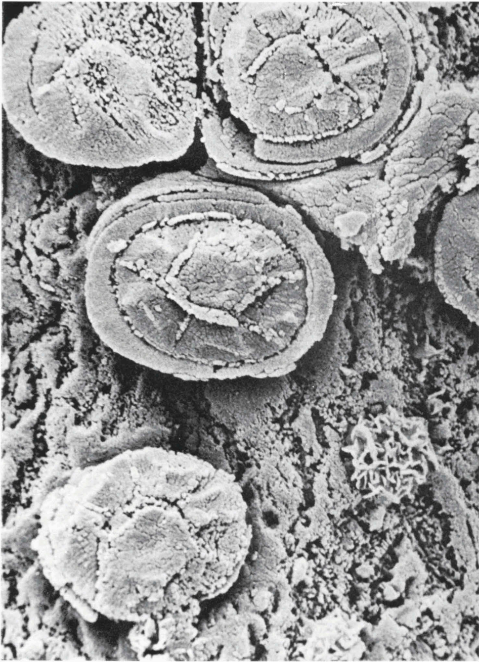
Fig. 18. Detail of Fig. 17: bordered pits showing radial structures in the margo, 3100 X, TFDL.
