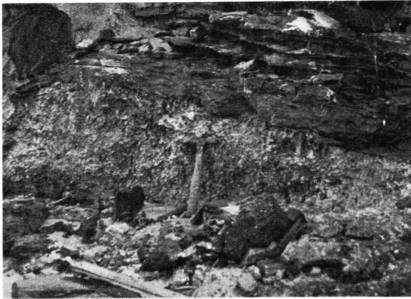
Fig. 52. Transition zone, against which the hammer is placed, stopping abruptly against the lignite containing sandlayer. Maria Elisabeth Mine (Mackenzie).
