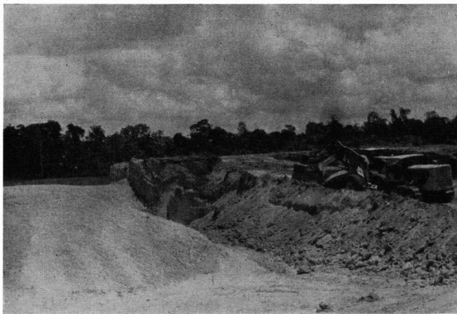
Fig. 54. Irregular surface of the bauxite-ferrite layer at Ituni, caused by old creekbeds.
