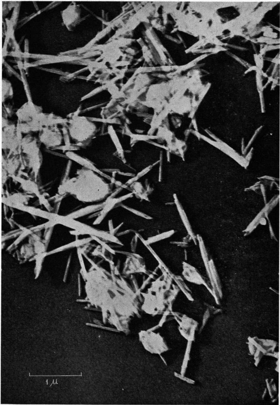
Fig. 81. Electron micrograph of the transition zone soil cover clay — bauxite showing metalloxyite and gibbsite, (Coropina formation, Onverdacht).
