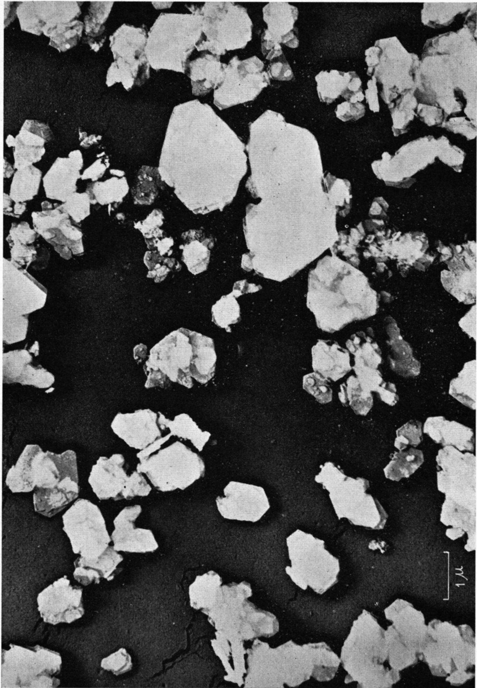
Fig. 69. Electron micrograph of autochthonous kaolin (Montgomery Mine, Mackenzie). Some kaolinite flakes show resorption; besides kaolinite, spatulae of splitted (meta)-halloysite are also seen.
