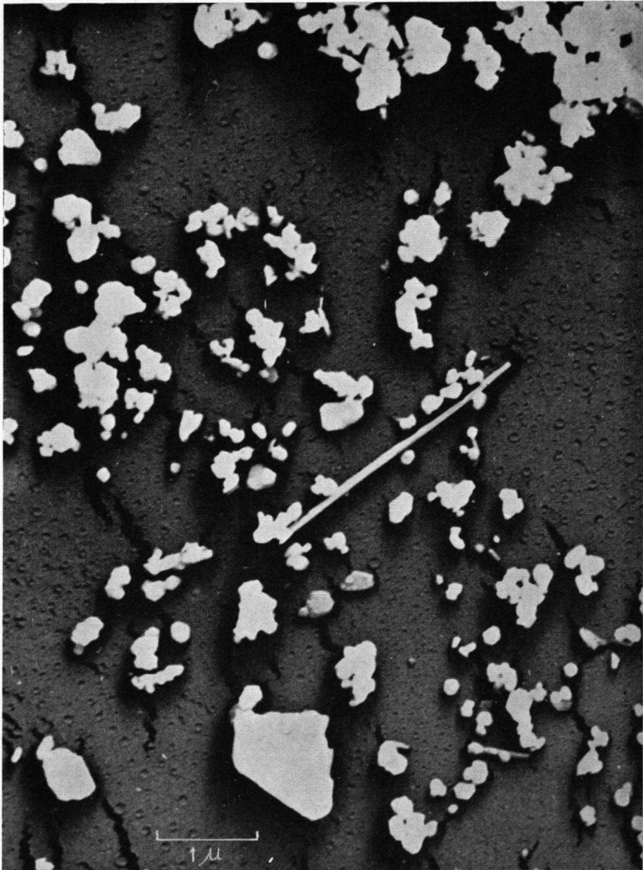
Fig. 83. Electron micrograph of a clay enclosure in bauxite (Onverdacht), showing kaolinite, metahalloysite and gibbsite.
