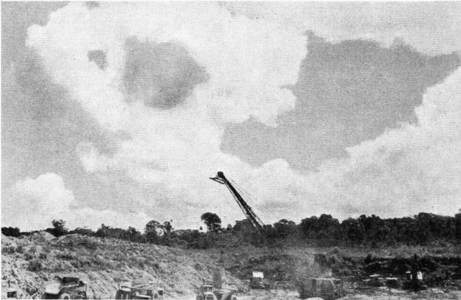
Fig. 42. Removal, with a mechanical shovel, of the swamp clay, which forms here the soil cover over the bauxite, which is removed with a dragline (Onverdacht).
