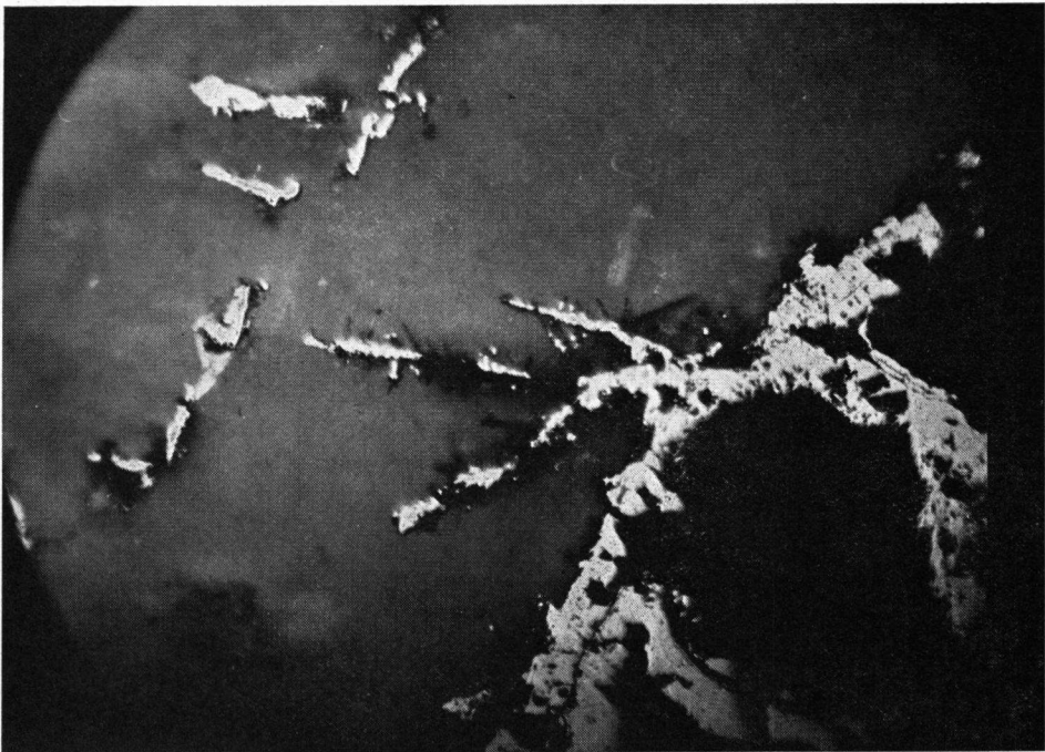
Fig. 62. Polished section of ferrite. In the kaolin, goethite penetrates and alters to hematite (Ricanau Hill). \times 85 .
