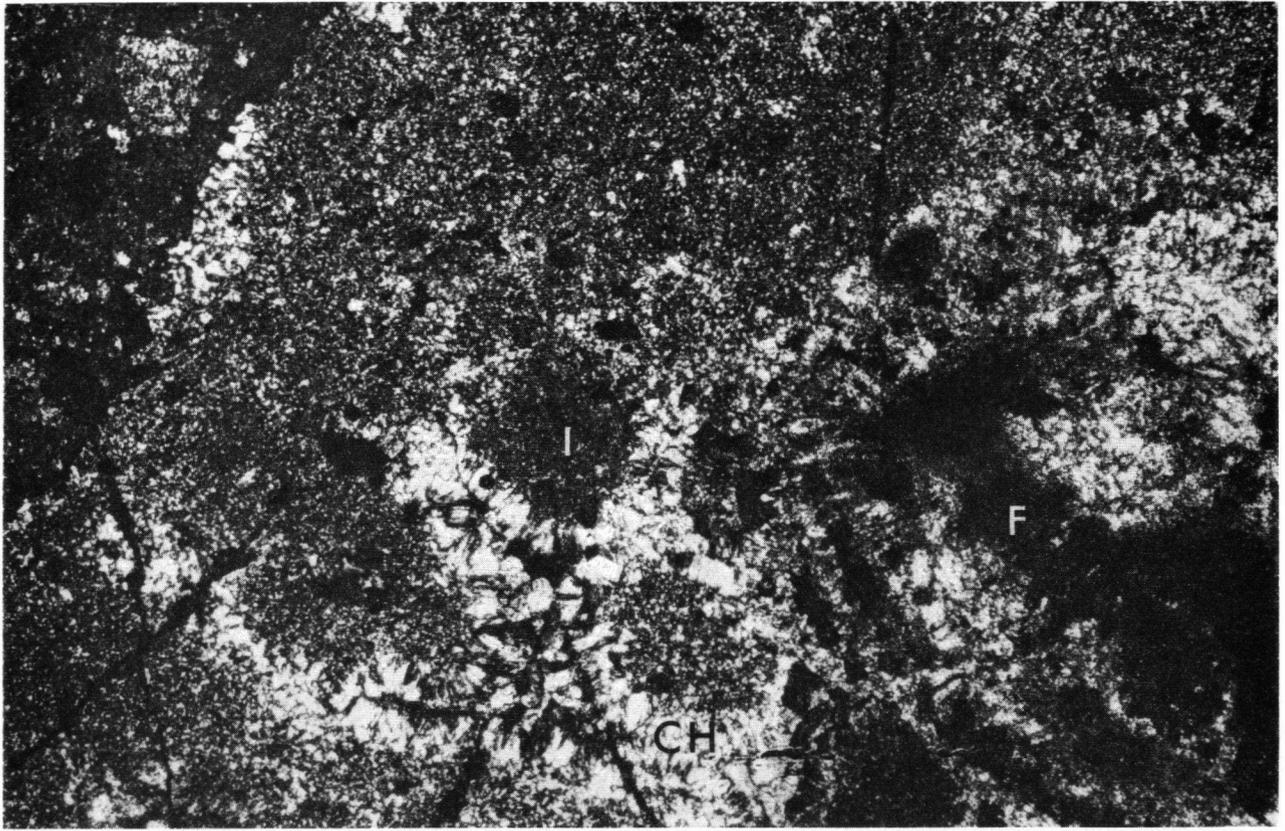
Fig. III-10. Chalcedony (CH) filling up pore spaces between clastic grains. Intraclasts (I) and fossil fragments (F) replaced by chert. 25 ×, crossed nicols.
