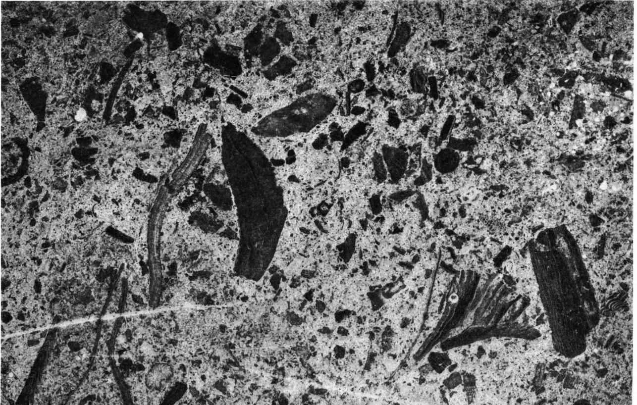
Fig. IV-9. Typical bioclastic limestone composed of fragmented rudists and micrite. Common lithofacies along the border of the Upper Cretaceous basin in the south-central Pyrenees. 8 ×.
