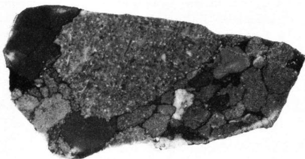
Fig. III-11. Stylolitic contacts between polymict limestone rock fragments in a breccia layer. Natural size.
