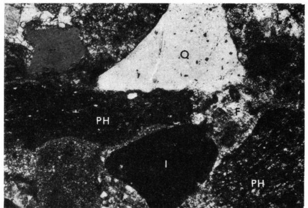
Fig. III-7. Calcareous phyllite fragments (PH) in a coarse-grained turbidite in which angular quartz grains (Q), fossils (F) and intraclasts (I) also occur. 25 ×.
