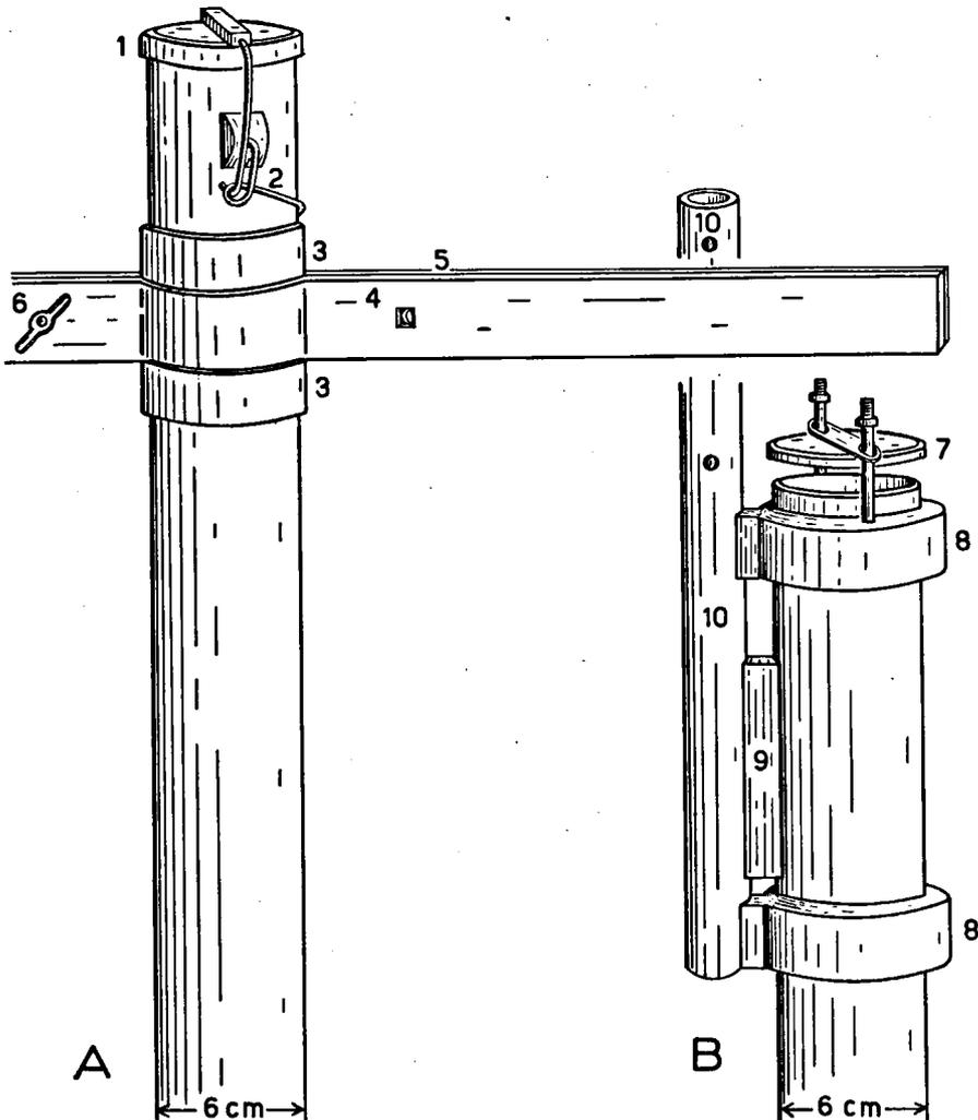
Fig. 22. Coring tubes. A: used on land and tidal flats; B: used for channel floors. 1,7. Brass lid with thick rubber plate; 2. Closing gadget; 3,8. Brass rings, soldered on tube; 4,5. Pair of iron bars, fitting around tube; 6. Winged nut, for fixing of bars; 9. Piece of brass to permit fastening of iron bars (4,5), when used for boring on land; 10. Hollow brass rod for fastening of first extension piece.
