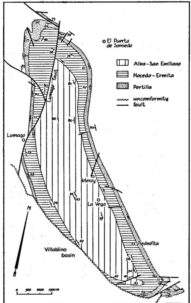
Fig. 93. The entire Palomas syncline and Lumajo fault. This figure shows that a deviation of the strikes occurs near the Lumajo fault and also that strike-slip movement took place along the Lumajo fault.
