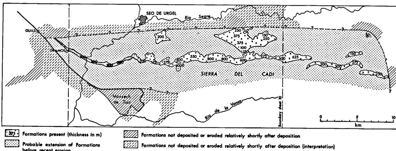
Fig. 18. Distribution and thickness of the Erill Castell Volcanics and the Malpas Formation.
