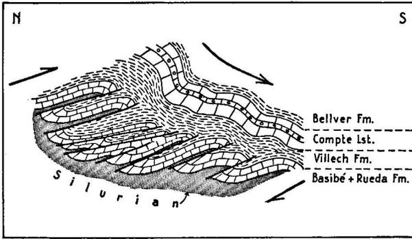
Fig. 44. Sketch section showing the thrusting in the Rueda and Basibé Formations and the related gliding of the Compte and Beller Formations.
