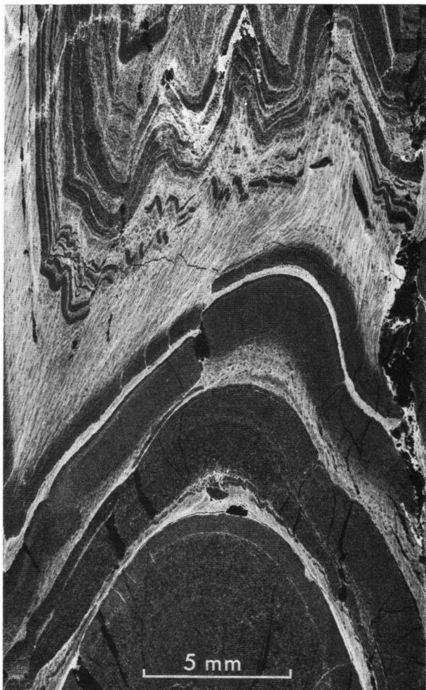
Fig. 31. Thin section showing mixed  $F_2$  folds and deviations of  $s_2$  in the Seo Formation (negative print).
