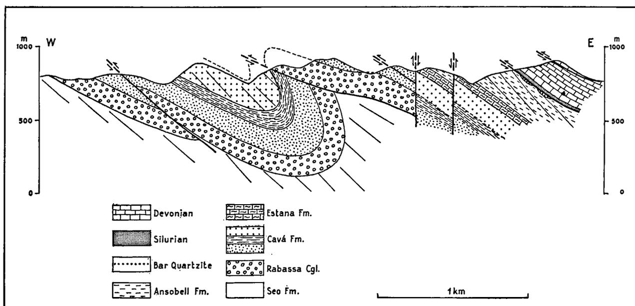
Fig. 35. E-W cross-section through the Cambro-Ordovician along the Segre valley between Seo de Urgel and Torres.
