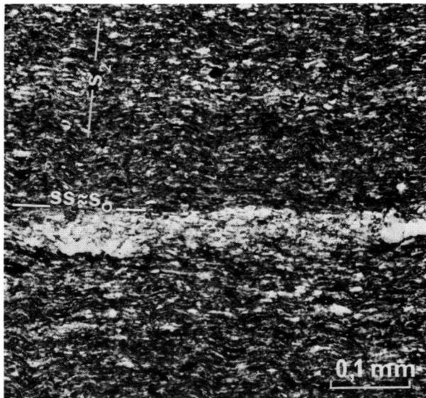
Fig. 26. Thin section of slates from the Seo Formation with slaty cleavage minerals statistically parallel with the bedding, gently crenulated by  $F_2$  deformation (crossed nicols).
