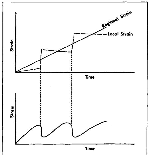
Fig. 54. Sketch diagram of stress-time and strain-time relationships.
