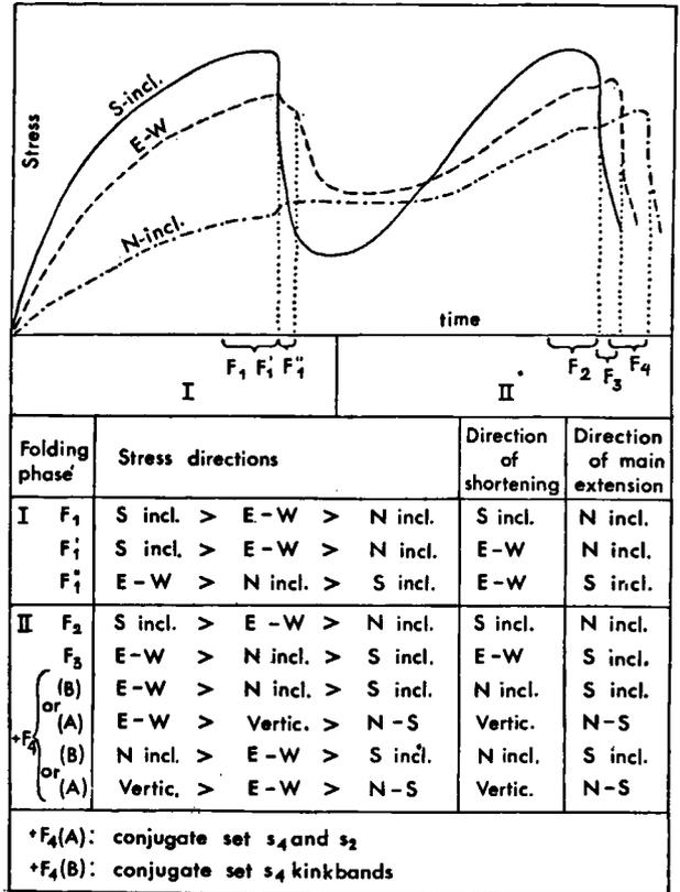
Fig. 55. Schematic stress-time diagram showing the relation between successive Hercynian deformation phases.
