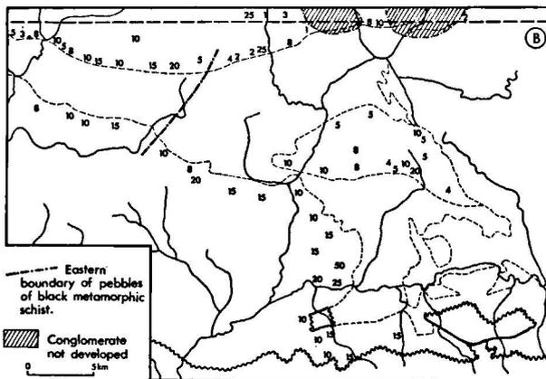
Fig. 4B. Distribution of maximum pebble size of the Rabassa Conglomerate (centimetres).
