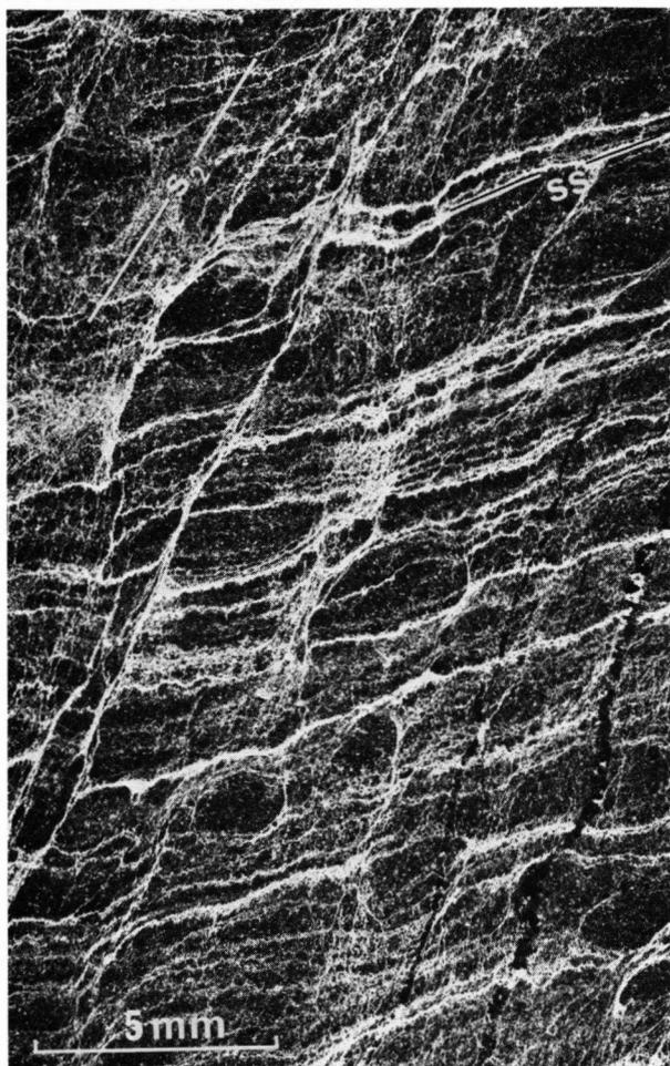
Fig. 28. Thin section showing  $s_2$  fracture cleavage in fine-grained sandstone of Civis Formation (negative print).
