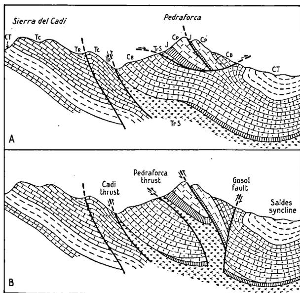
Fig. 60. Cross-sections showing two different interpretations of the Pedraforca structure: (A) according to Guérin-Desjardins & Latreille (1961), (B) according to the present author.
