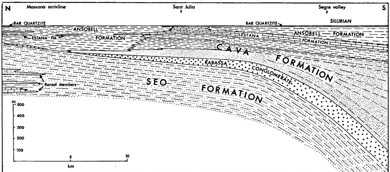
Fig. 9. Schematic N-S cross-section through Cambro-Ordovician formations.
