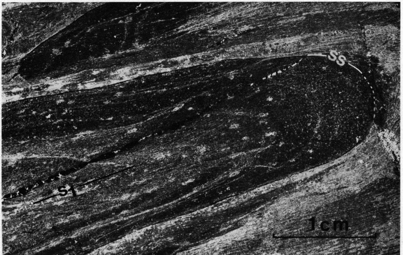
Fig. 26. Micro-photograph of isoclinal s_1 -fold with accompanying axial-plane slaty cleavage; enlarged directly from thin section.
