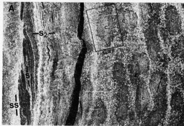
Fig. 28A. Thin section showing bedding, s_1 - and s_2 -cleavages, and contact metamorphic cordierite crystals enclosing both these cleavages (enlarged directly from thin section).
