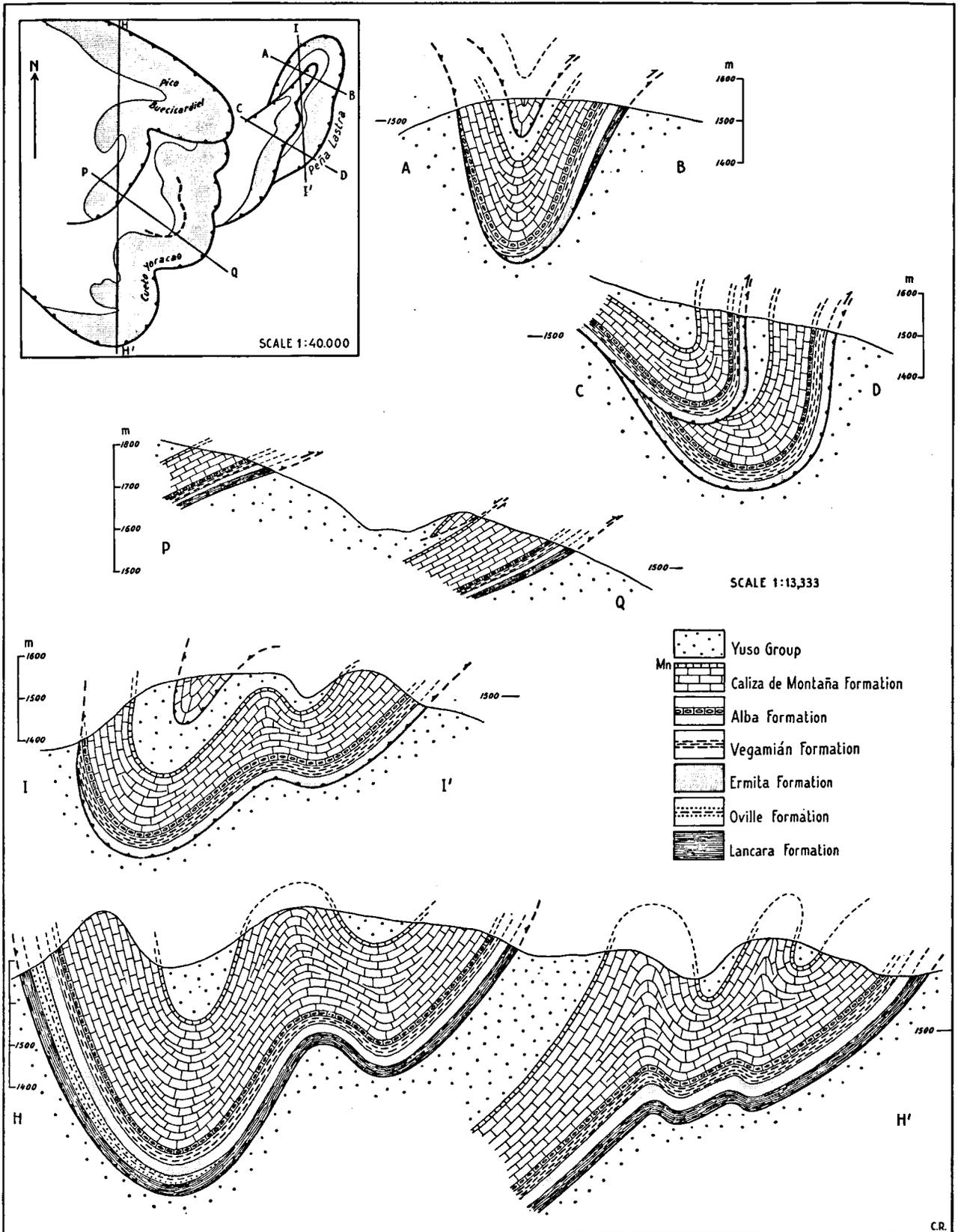
Fig. 55. Structural sections showing cross-folding in the Fontasguera subarea.
