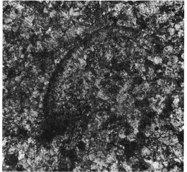
Fig. 25. Caliza de Montaña Formation; biomicrosparticle, the shell and its surroundings unaffected by recrystallization. (100  $\times$ )
