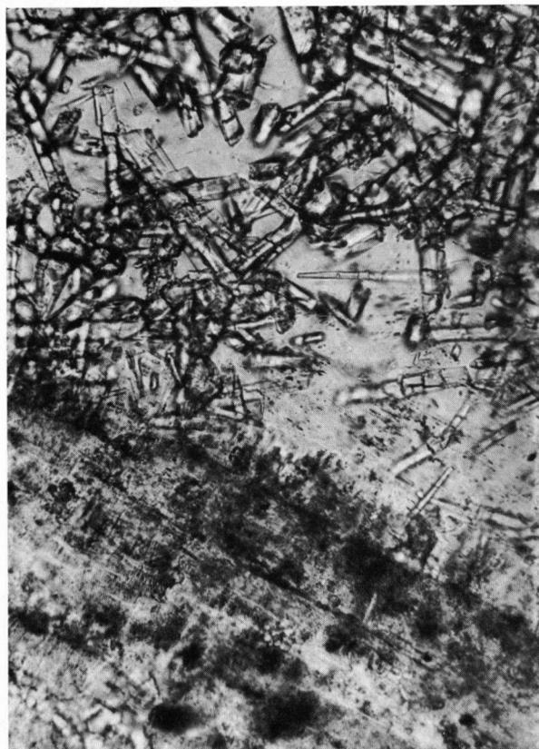
Fig. 61. Dolerite; regeneration of basic feldspar giving rise to fresh and glassy feldspar (albite-oligoclase) with enclosed epidote. (250 ×)
