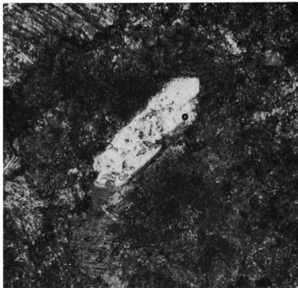
Fig. 7. Lancara Formation, limestone-dolomite member; authigenic bipyramidal quartz crystal. (100  $\times$ )
