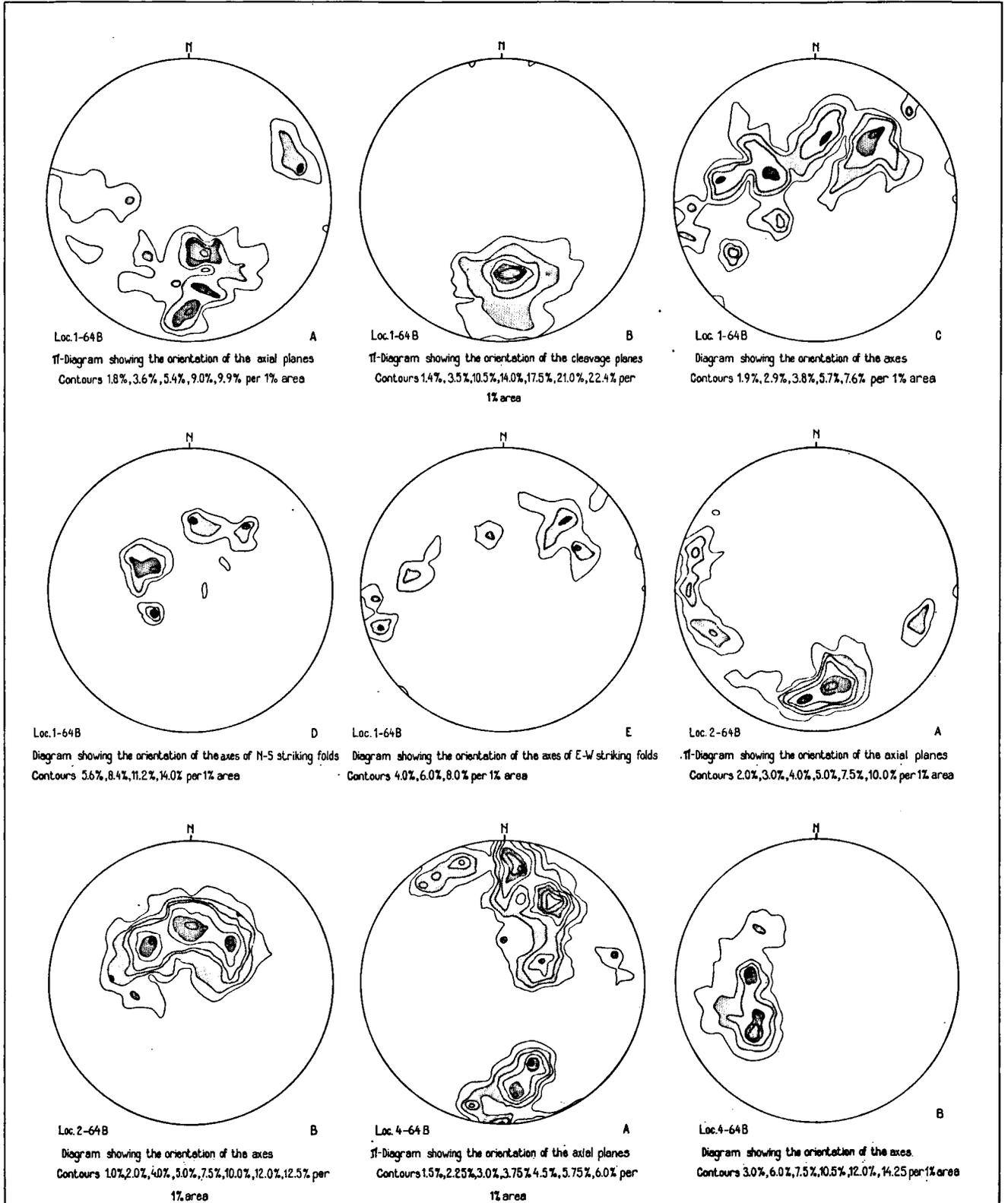
Fig. 52. Orientation of the axial planes, cleavage planes, and axes of Hercynian folds.
