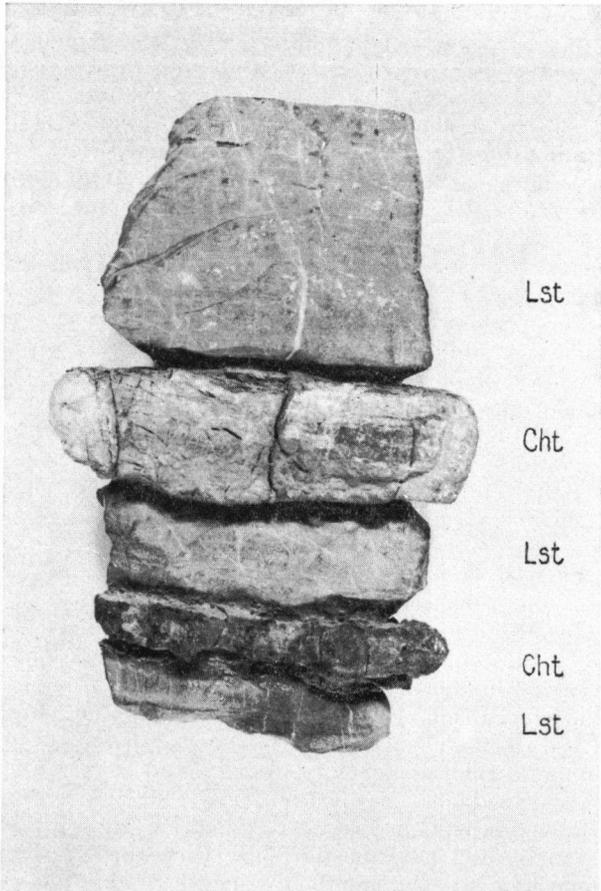
Fig. 24. Caliza de Montaña Formation; alternation of thin chert and limestone layers. (natural size)
