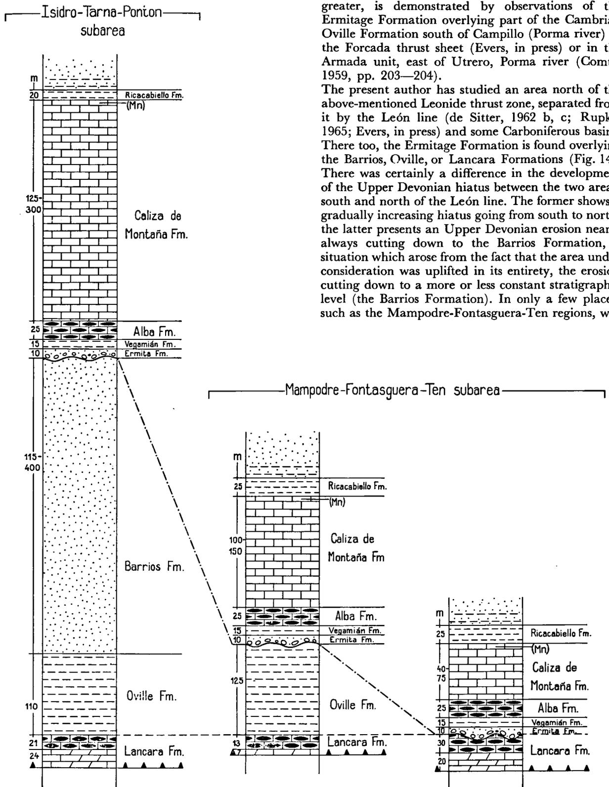
Fig. 14. The Upper Devonian Ermita Formation in unconformable contact with various older Paleozoic rock-stratigraphic units.
