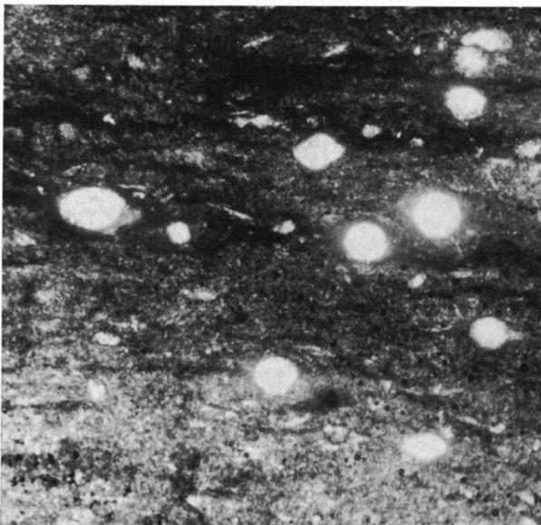
Fig. 23. Alba Formation; radiolarian chert with circular and elliptical radiolaria. (40 ×)
