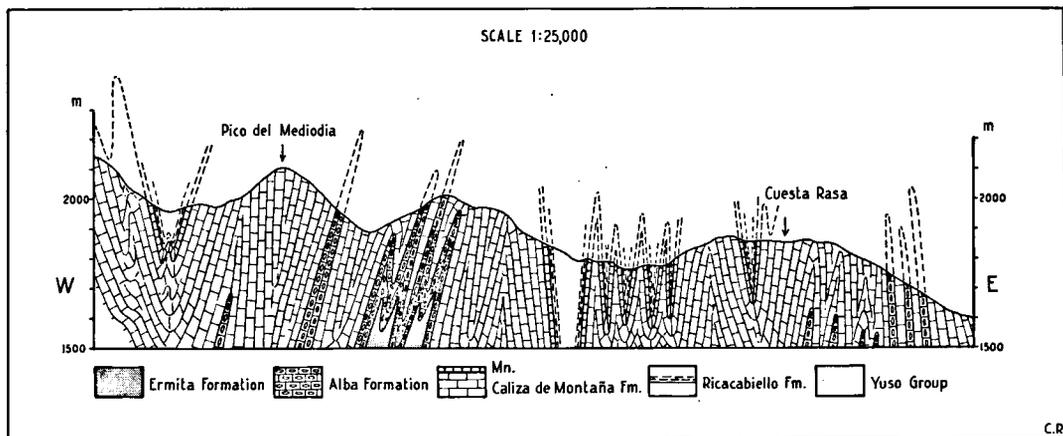
Fig. 53. Structural section through the Mampodre subarea.
