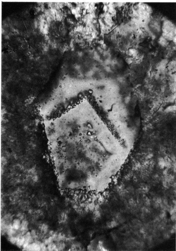
Fig. 10. Lancara Formation, limestone-dolomite member; authigenic quartz crystal with carbonate inclusions showing successive stages in the development of the authigenic material. (420 ×)
