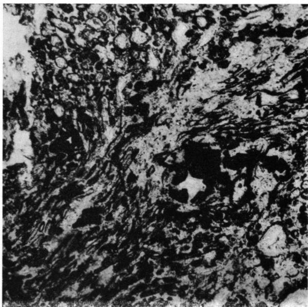
Fig. 62. Pyroclastic rock; flow-structures caused by stretching and a parallel arrangement of leucoxene concentrations and spherulites. (100 ×)
