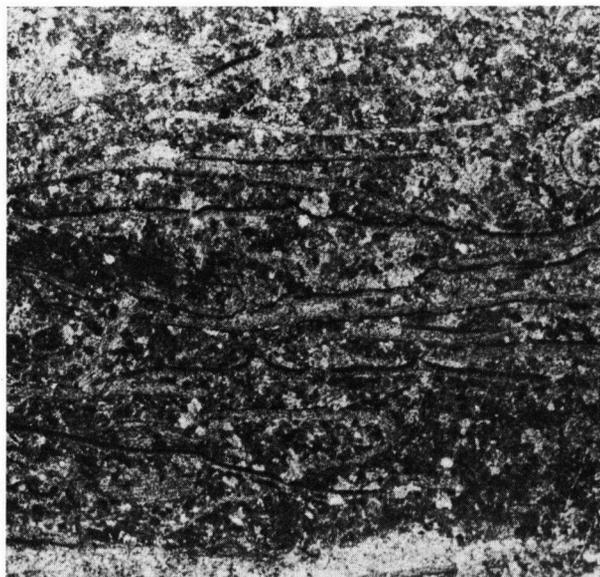
Fig. 6. Lancara Formation, limestone-dolomite member; trilobite biomicrite with trilobite fragments concentrated in the bedding plane (section taken perpendicular to the bedding plane). (15  $\times$ )
