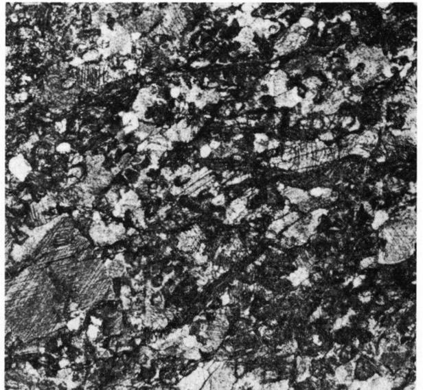
Fig. 26. Caliza de Montaña Formation; intrasparite, partly recrystallized. (10  $\times$ )
