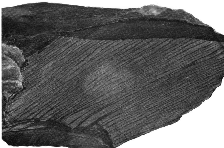
Fig. 6 Fracture cleavage in quartzitic layer in phyllite; detail of fig. 5 ( 1\times )
