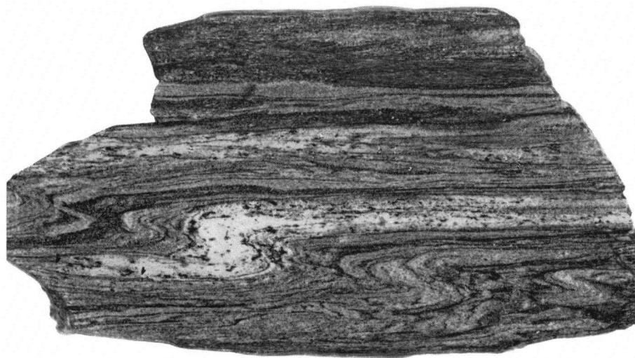
Fig. 7 Folded bedding with axial plane schistosity s_1 in micaschist. (1 ×)
