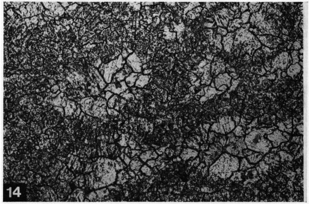
Fig. 15. (Specimen 32B). Laminar specimen with transversely fibrous tissue. Microlamination not completely disappeared. Tissue borders irregular. (vert. section)  $\times$  57.
