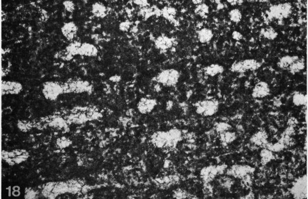
Fig. 19. (Specimen 61). Melanospheric specimen with pigment concentrated around galleries (below) or in the vertical structure elements. Some galleries are also partly or completely filled with pigment. Microlaminae visible as clear bands. Intergrown with *Syringopora sp.* (vert. section) × 57.
