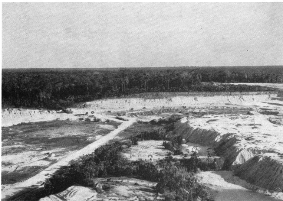
Fig. 22. Bauxite mine near Kwakwani. In the mine face the overlying sands of the Mackenzie formation are visible. (Photograph taken from the air).
