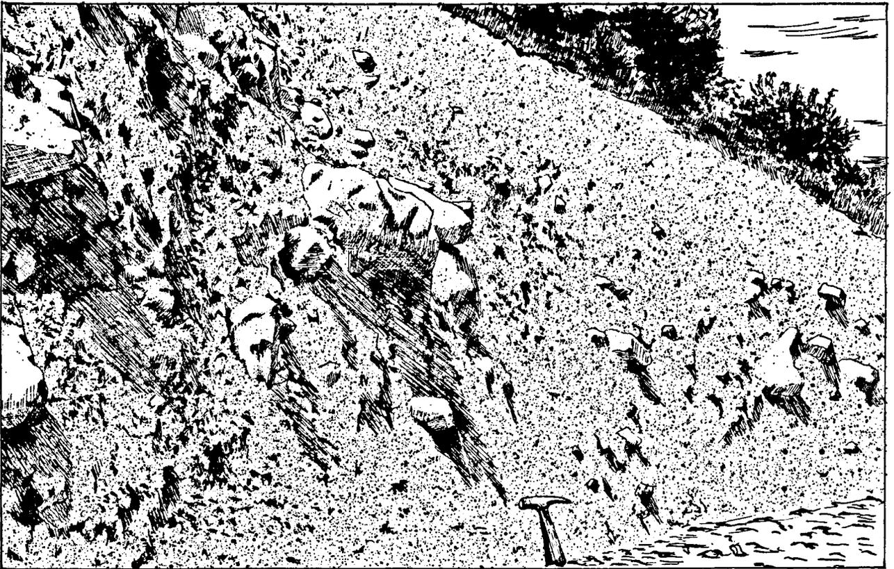
Fig. 10.2 Fluvio-glacial material in the left Aiguamoix bank at the dam axis (elev. 1400 m).
