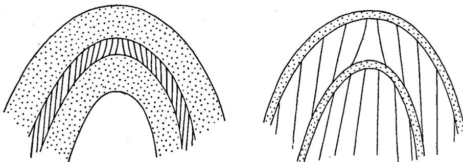
Fig. 3. Development of cleavage in thick and thin slates between competent beds.
