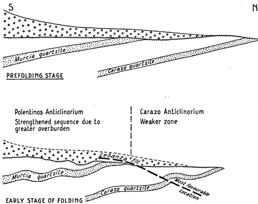
Fig. 38. The development of the Lebanza thrust at the pre-Yuso unconformity.
