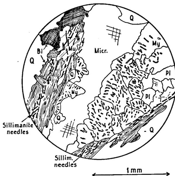
Fig. 9. Myrmekite replacing potash-felspar.
