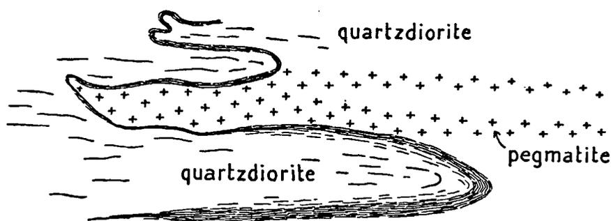
Fig. 30. Saddle reef of pegmatite which is still connected with parallel pegmatite bands in the quartz-diorite. Scale 1: 50. (lunch tree).
