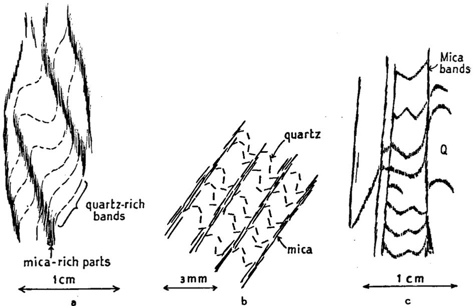
Fig. 5. Mica-schists showing different stages of the development of  $S_2$  which cuts obliquely through an older banding.
