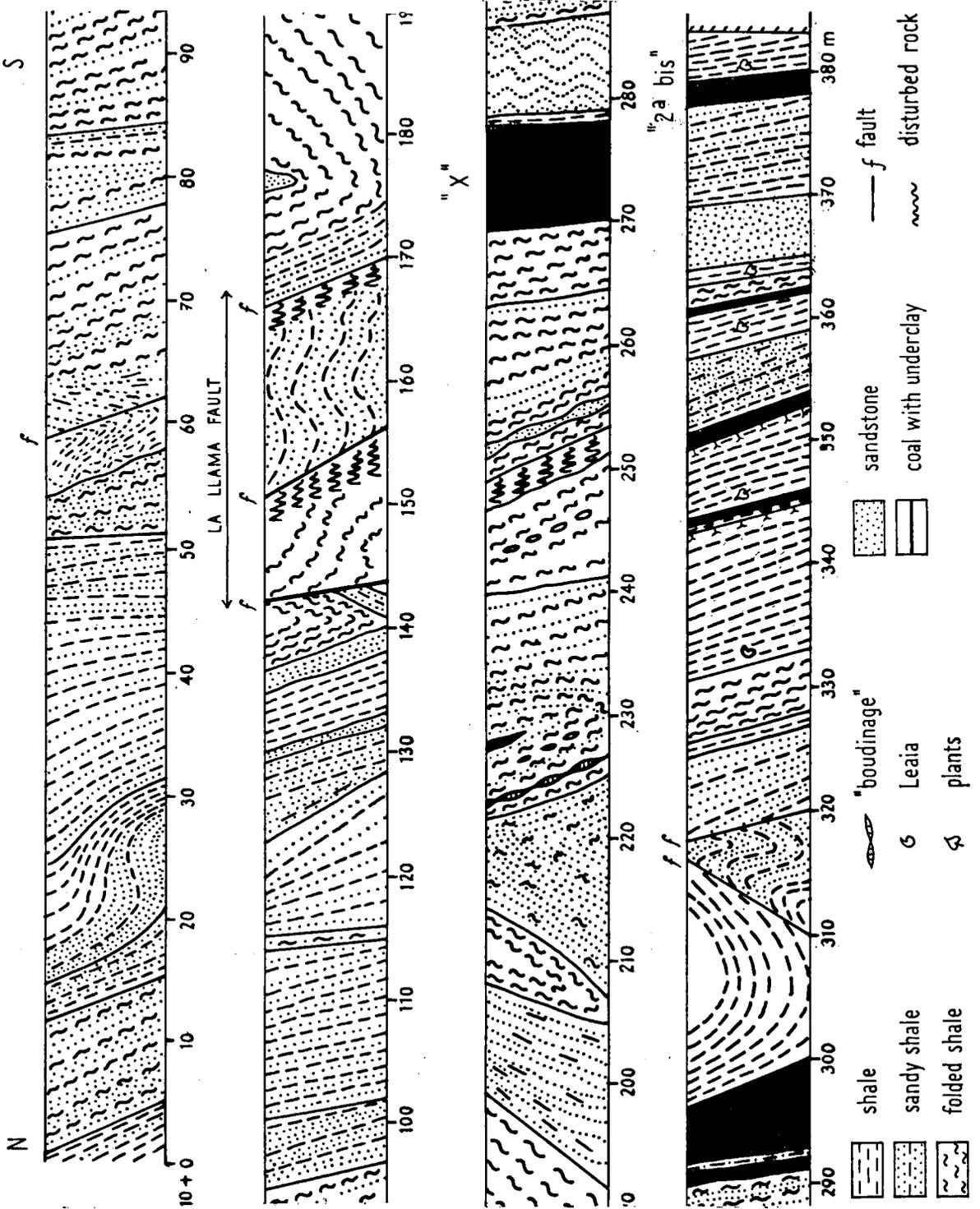
Fig. 29. Section in the cross-cut 3W—7mo Recorte (approx. 180 m below surface) of the Sotillos colliery, showing thrust faults.
