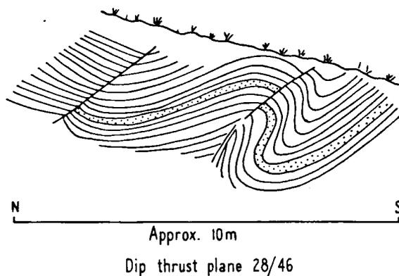
Fig. 23. Subsidiary structures of the southern branch of the Valderrueda fault system (occurring just south of the fault, about 1 km east of Taranilla).
