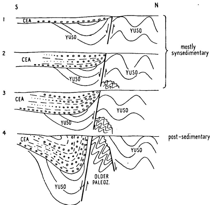
Fig. 26. Schematic representation of the development of the Tejerina syncline.
