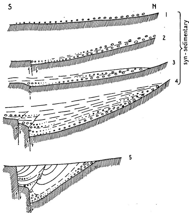
Fig. 30. Schematic representation of the development of the Sabero syncline.
