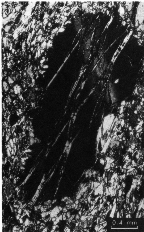
Fig. 3. The chlorite peridotite mylonite, strained olivine porphyroclasts embedded in recrystallized matrix grains.
