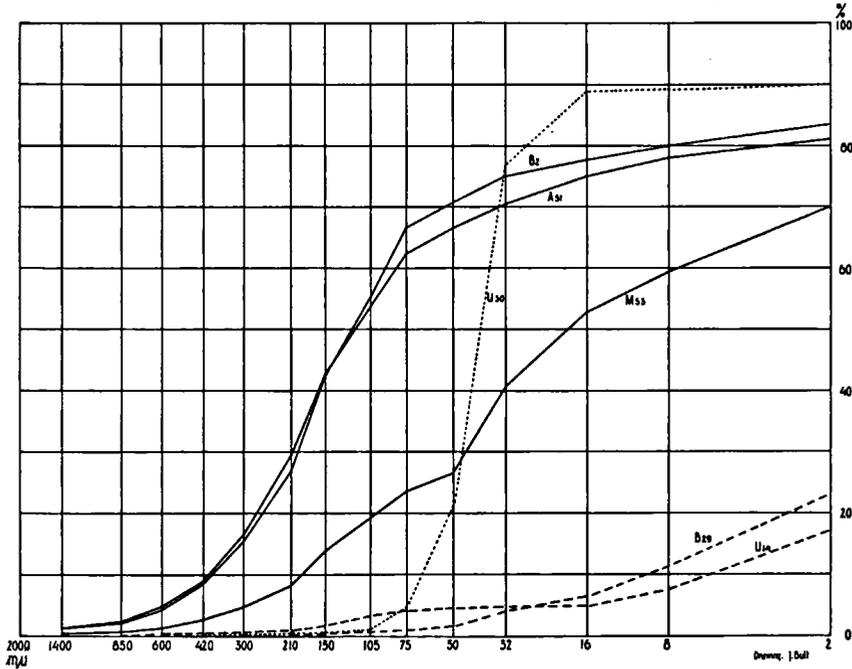
Fig. 3. Grain size diagram of investigated sediments
