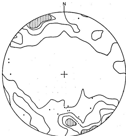
Fig. 5. Equal-area projection of 202 fold axes of minor recumbent folds from an area of paragneisses east and northeast of Complex (contours), and of 16 fold axes of minor folds in inclusions in Complex (dots). Contours 5-4-2-0.5 % per 1 %-area.
