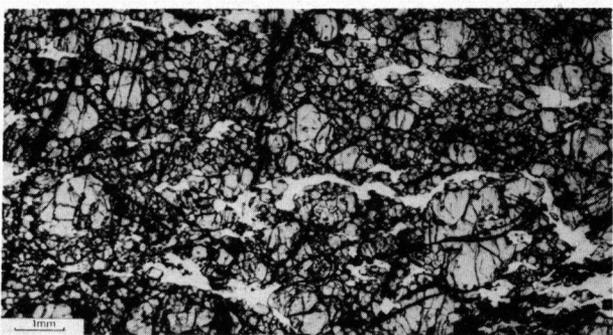
Fig. 4. Garnets, larger grains, in mosaics of recrystallized clinopyroxene. Thin section RGM 129088.
