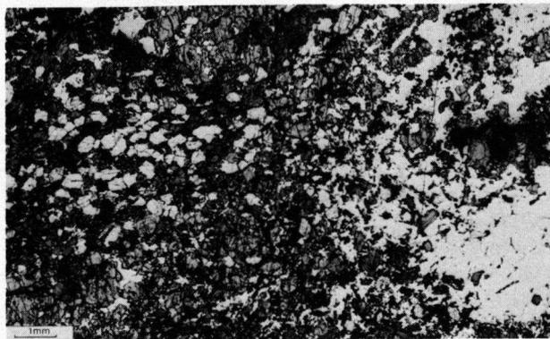
Fig. 11. Granoblastic scapolite-bearing gneiss. White grains on the left are epidotes, white mosaics on the right contain scapolite. Garnets, light grey; clinopyroxene, dark grey. Thin section RGM 129103.
