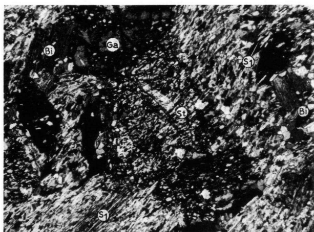
Fig. 2.2. Staurolite (St), biotite (Bi) and garnet (Ga) crystals cutting across S_1 cleavage defined by muscovite in Tower Hill area 40 \times .
