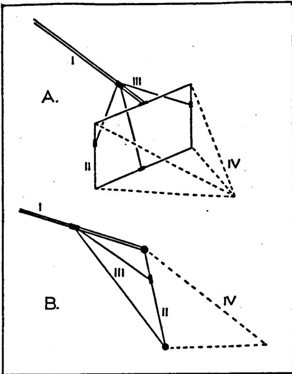
figure 1.1. The sample net as it was used to catch prey. (A). 3-Dimensional view. (B). side view. (I) Handling stick. (II) Window frame (80 x 40 cm). (III) Support rods. (IV) net.
