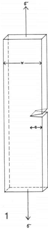
Fig. 1. Opening mode (Mode I) of crack propagation for a single-edged-notched specimen.
