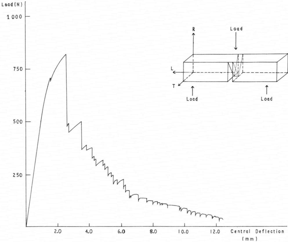
Fig. 3. The load-deflection curve obtained from a work of fracture measurement of wood in three point bending. The diagram in the top right illustrates the testing geometry.
