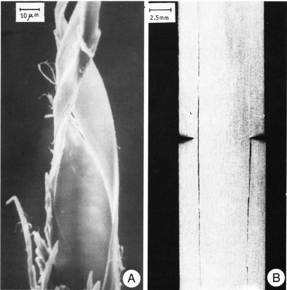
Plate 1. — A. Tensile failure of Sitka spruce. The post-buckling aspect of a tracheid showing the characteristic spiralling cracks (SEM photograph).—B. Cook & Gordon mechanism at the tip of a crack. Sitka spruce strip loaded in tension.
