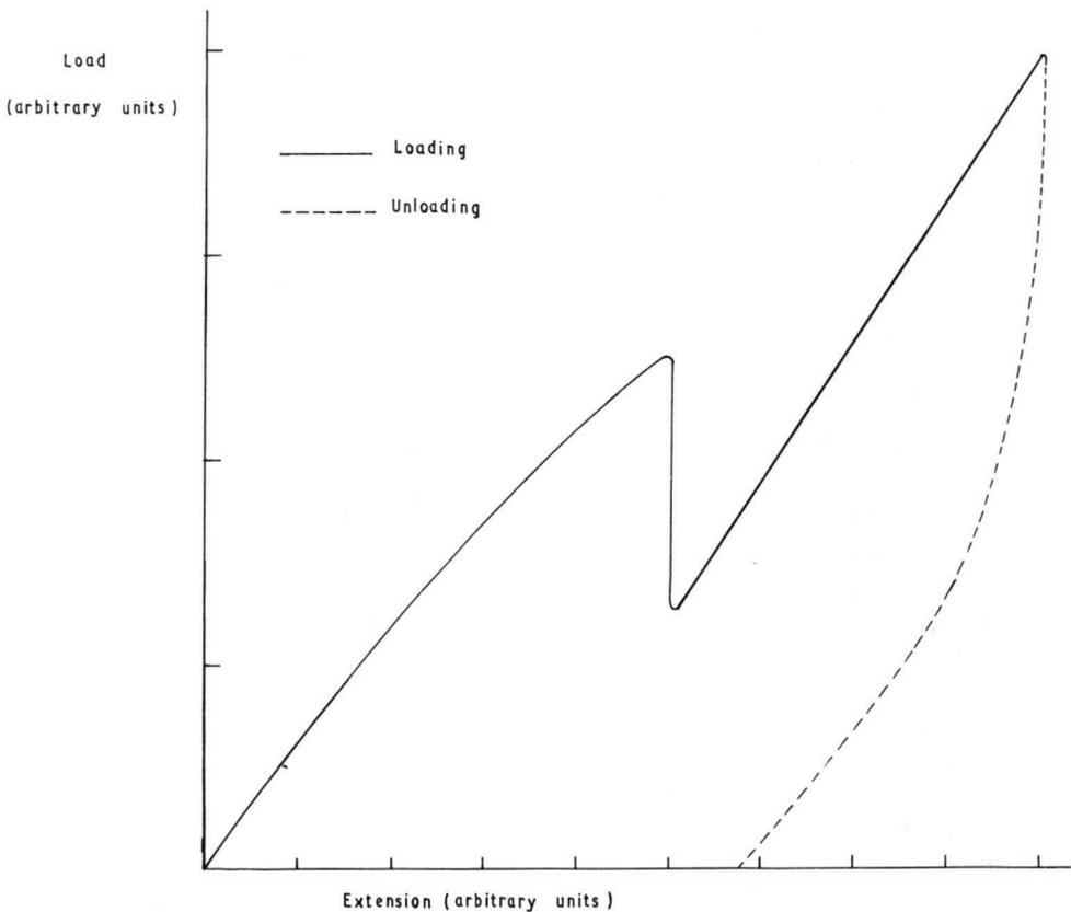
Fig. 4. Load-extension curve for a hollow helically wound tube of glass fibre and epoxy resin.
