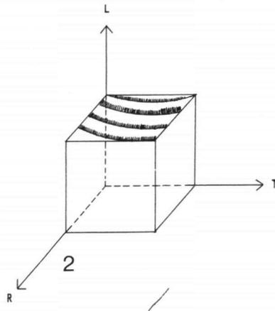
Fig. 2. Reference system for crack propagation in wood.
