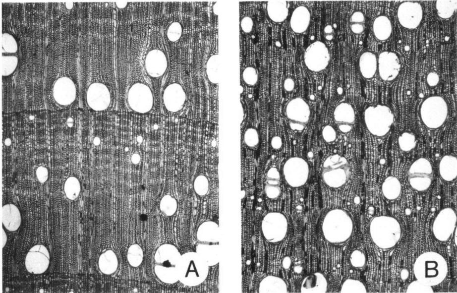
*Plate 1.* The influence of rate of growth on fracture morphology and toughness of hickory. Sample A had a growth rate of 14 rings per 25 mm, a density of 780 kg/m<sup>3</sup> and in the Hatt-Turner toughness test the height of drop was 2 m. The corresponding values for sample B were 30 rings per 25 mm, 630 kg/m<sup>3</sup> and only 0.70 m.
